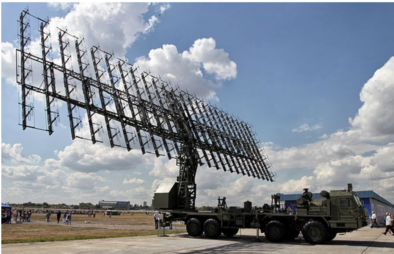
Fig. 1: Large planar array antenna of a VHF Russian mobile air defense radar, the Nebo-M. It consists of 175 folded dipole antennas driven in phase. It radiates a narrow beam of radio waves perpendicular to the antenna. By Vitaly V. Kuzmin , CC BY-SA 4.0
